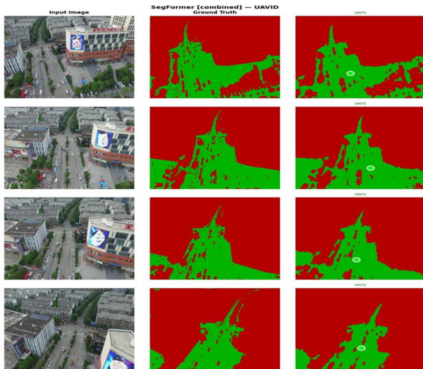
Figure 5: SegFormer combined results on UAVid; the predicted centroid (White Circle) lands inside a ground-truth safe region in 78.4% of test images, and the model reliably picks roads over rooftops in dense urban scenes.
